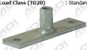
An extra thick, extra long (XL) two-hole bracket used for Concrete and Masonry connections in conjunction with 12mm Concrete Screw Bolts. Can also be fixed with conventional nylon plug & coach screw, with threaded studs or sockets set in resin or with bars or bolts, nuts washers etc passed right through the structure. Designed with hole centres of 150mm to spread the load over three courses of brickwork or to align with mortar joints.
