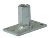
A mild steel bracket, with an M16 female thread reception, used to make connections to Timber or Steel. With six - 6.0mm holes at 70mm centres, they can be fixed with chipboard screws, woodscrews, coach screws, self-drilling screws or even riveted or bolted directly to or through the structure.
